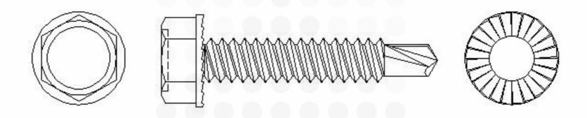
UNSLOTTED INDENTED HEX PRESSED WASHER HEAD WITH 24 LOCKING SERRATIONS UNDER THE HEAD SELF DRILLING SCREWS
