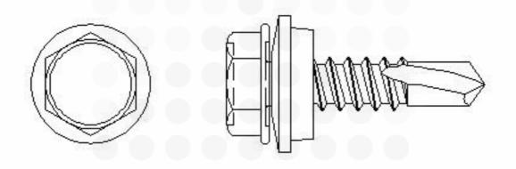
INDENTED HEX WASHER HEAD WITH UNDERCUT SELF DRILLING SCREWS WITH OD EPDM BONDED WASHER
