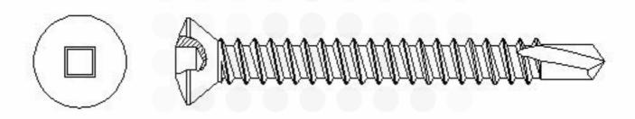
SQUARE SOCKET RECESS COUNTERSUNK OVAL HEAD SELF DRILLING SCREWS
